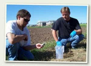
Spray into a measuring container for that amount of time. The number of ounces collected can be converted directly to GPA (Example: Collected 40 ounces from nozzle in 92 seconds, which equals 40 GPA).
