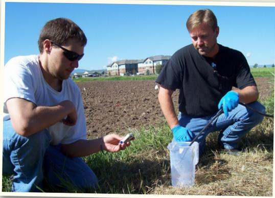
Spray into a measuring container for that amount of time. The number of ounces collected can be converted directly to GPA (Example: Collected 40 ounces from nozzle in 92 seconds, which equals 40 GPA).
